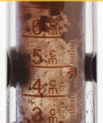
The DipTube uses principles of density and transparency to characterise the fuel inside your storage tank.
